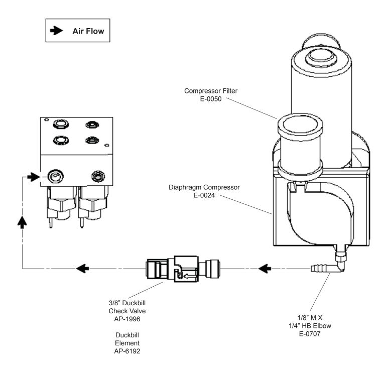
FIGURE 9 - Versa Trac Power Unit Internal Air Components
