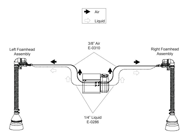
FIGURE 4 - Versa Trac Liquid and Air Flow
