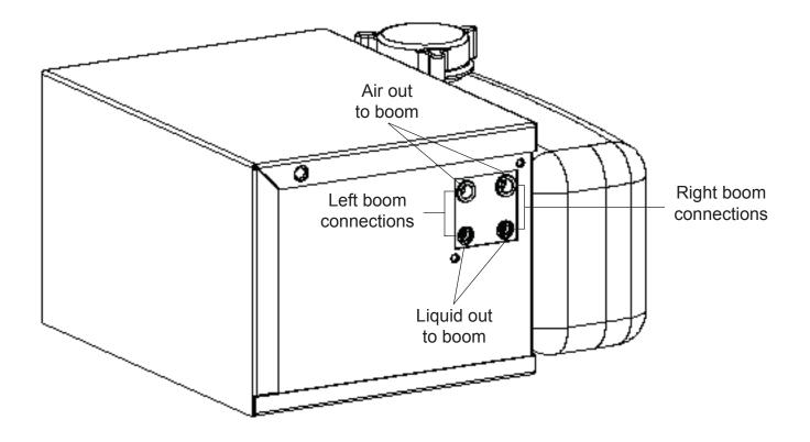
FIGURE 6 - Versa Trac Air/Liquid Connections
