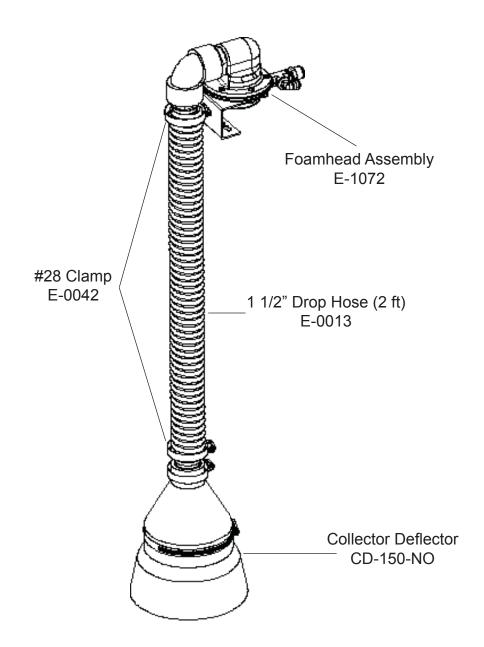
FIGURE 2 - Versa Trac Foamhead and Boom End Assembly
