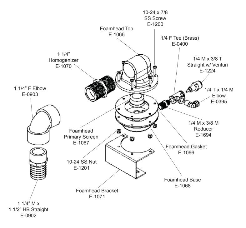
FIGURE 3 - Versa Trac Foamhead Assembly
