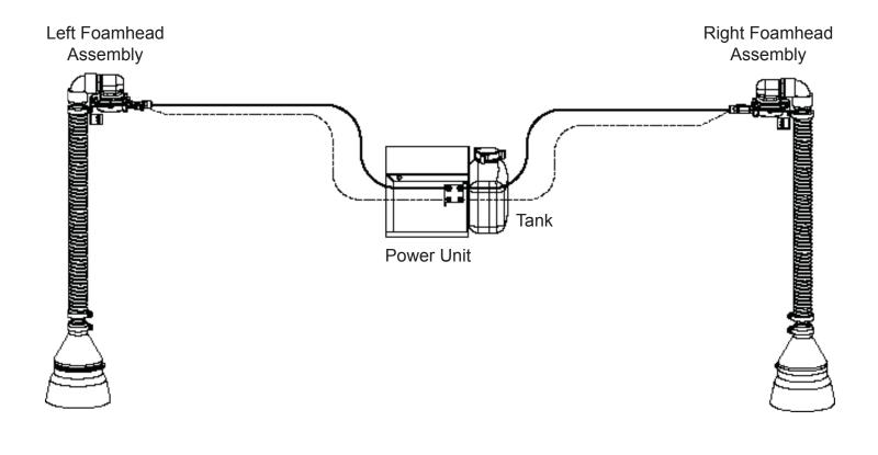
FIGURE 1 - Versa Trac Model VTD-2010 Foam Marker
